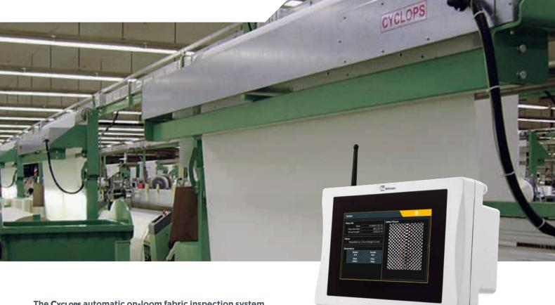
The CYCLOPS automatic on-loom fabric inspection system detects warp, filling and point defects by means of a moving camera system installed on the off-loom take up.
